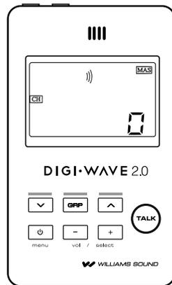
Must be set to Repeater, CH 0 and MAS. NOTE: For more than one repeater, repeaters on additional channels must be SLV.
