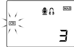
Channel icon will now begin to blink. Press (+) or (-) button to select a Channel number 1 – 14. Transmitting Channel must be set different. (N/A with Main Speaker unit. Set to CH 0).
