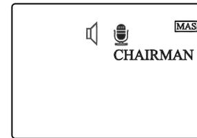
When mode selection is made MAS (for example) will blink (shown in screen 8). There **MUST** be **one** Master per group.
