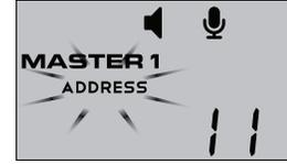
The ADDRESS icon will be blinking. Use the buttons then the button to choose address (0-1023).
