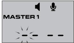
The first secure code digit will be blinking. Use to adjust the first digit.
