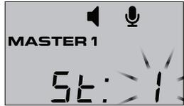
The Sidetone Level will be blinking. Use the buttons then the button to choose the Sidetone Level.
