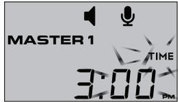
The TIME icon will be blinking along with the minutes. Use the buttons to adjust the minutes.
