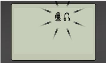
You are now at the beginning of the setup mode. To save and exit setup, hold NO and YES buttons together for 2 seconds
