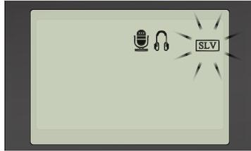
When mode selection is made SLV or MAS icon will blink. ( Receive only will not have this option. Skip to step 9 )
