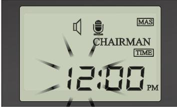
The hour number ( TIME ) will now blink. Press ( + ) or ( - ) button to select Hour number ( If unit is set as SLV or SLV CHAIRMAN, skip to step 19 ) **NOTE: Only CM sets time, SLV units auto-sync**
