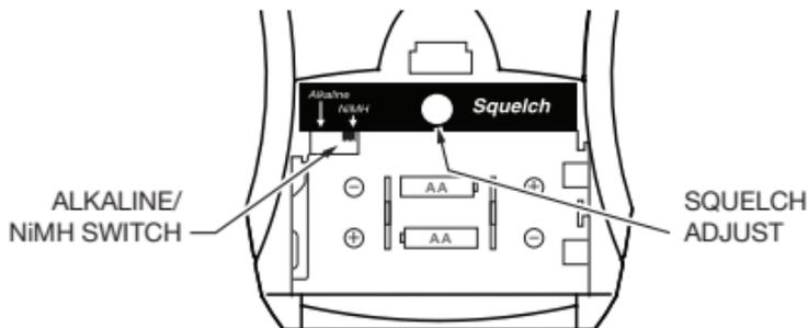
3. Insert 2 AA batteries over the fabric strip. Note correct polarity (+/-).
